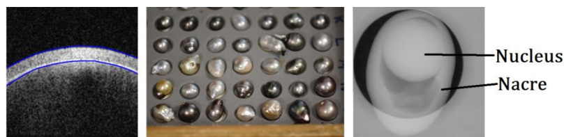
Fig. 3. One result image of the nacre thickness measurement from [1] (left), several Tahitian pearls with 'a baroque' shape prepared for X-raying (middle) and an X-ray image of a typical Tahitian 'baroque' pearl (right).
