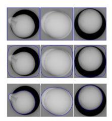
Fig. 4. The initial snake contour for the outer boundary detection in blue (top), after several iterations (middle) and the final result (bottom).
