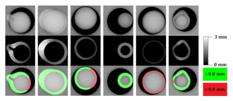
**Fig. 8.** Original images (top), automatically calculated nacre profiles (middle) and a visualization of areas lower than the minimal allowed nacre thickness for exporting a Tahitian pearl (bottom, areas lower than 0.8 mm in red).
