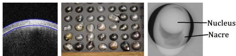
**Fig. 3.** One result image of the nacre thickness measurement from [1] (left), several Tahitian pearls with 'a baroque' shape prepared for X-raying (middle) and an X-ray image of a typical Tahitian 'baroque' pearl (right).
